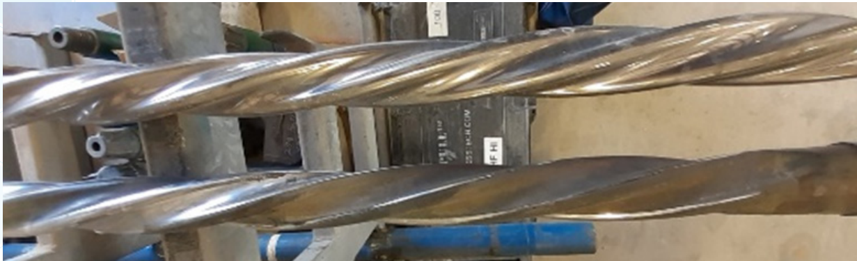
Figure 3: Motor after contact with HCR-7000-WL (top) and 15% HCl (bottom).
