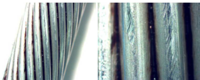
Figure 1. Surface of the greased wireline cable prior to acid testing at 10X magnification (left) and 40X magnification (right).
