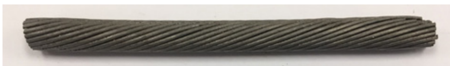
Figure 1. Wireline after exposure to 1:2 Enviro-Syn HCR-7000FRAC-WL at 90°C (195°F) and 2,750 kPa (400 psi) for 120 hours.
