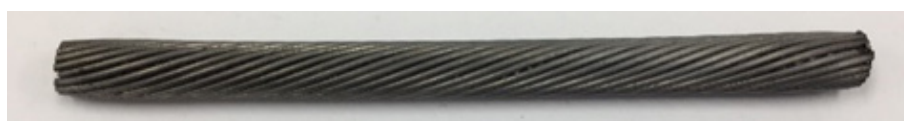
Figure 1. Wireline after exposure to 1:2 Enviro-Syn HCR-7000-WL at 90°C (195°F) and 2,750 kPa (400 psi) for 120 hours.
