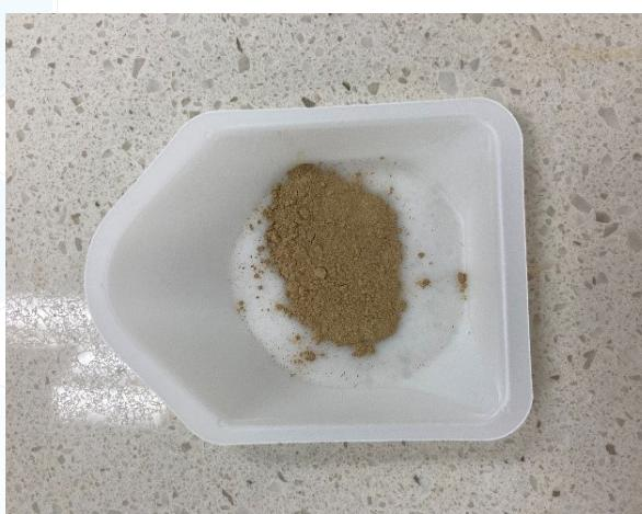
Figure 1. Scale sample from West Africa offshore well.
