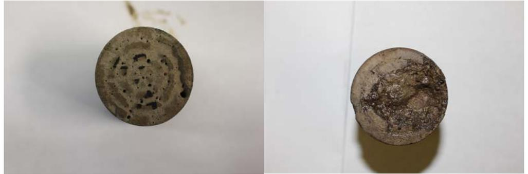
Note: Wormholing seen on HCR core compared to severe face dissolution on HCL treated plug
